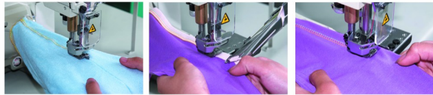
倒骨缝 Inverted seam 滚领缝 Roll Neck Seam 下摆缝 Hem seam
